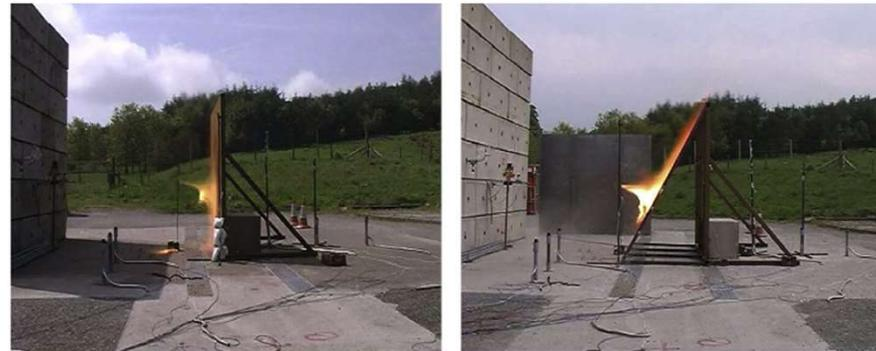
Photos of the release location and vertical wall (left) and 60° barrier (right) also shown in the resulting jet fire images
