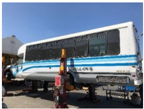
Bus being converted to fuel cell power
