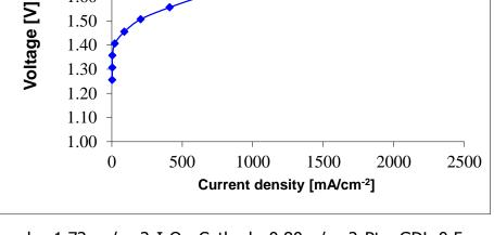
Anode: 1.72mg/cm2  $IrO_{2,}$  Cathode 0.80 g/cm2 Pt, GDL 0.5mm Ta coated steel felt, Aquivion membrane, 60 microns thick, Temperature 120°C, Pressure 3 bar
