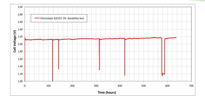
Life test (> 600 h) obtained with the ACTA alkaline MEA 475 mA/cm<sup>2</sup>),  $T_{cell} = 40$  ° C. Now more than 6000 h!
