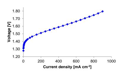
Anode: 0.98 mg/cm2 IrO<sub>2</sub>, Cathode 0.34 g/cm2 Pt, GDL 0.5mm Ta coated steel felt, Aquivion membrane, 63microns thick,
