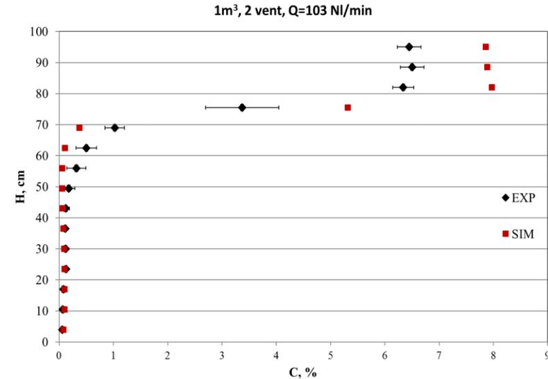
→ CFD results in good agreement with the exp measurements (exp error is of 3%)
