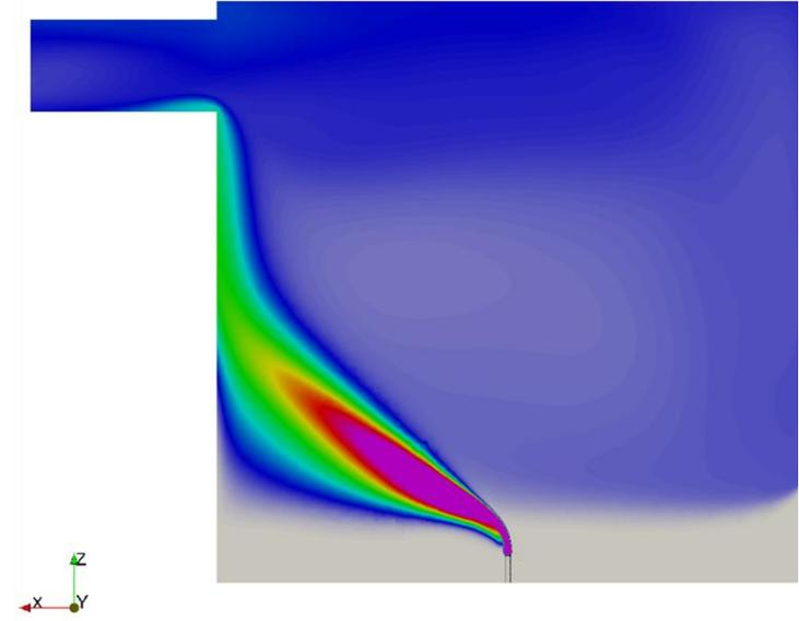
According to ventilation, the jet seems directly oriented in the outlet flow, induced by the ventilation, without mixing with the other parts of the enclosure...
