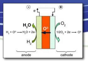
SOFC and PCFC drawbacks: water at anode (SOFC) or cathode (PCFC)
