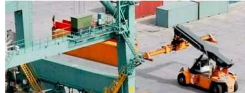
Reach Stackers are used to handle containers and other cargo in ports; they are both able to shortly transport as well as to pile containers
