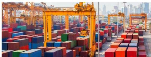
**Brief description** Rubber tyred gantry (RTG) cranes are mobile cranes which are used to ground or stack containers from yard tractors or drayage trucks and vice versa
