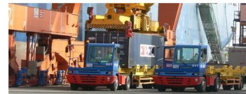
Yard tractors are used to transport trailer and containers short distances from ships to distribution centres or container terminals and vice versa
