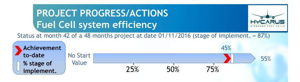
For our target application (Generic Fuel Cell System), maximum efficiency operating point is 55% of rated power. Corresponding target efficiency is 46% under airborne operating conditions (low ambient pressure for example).
