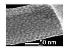
Thin Pt islands formed by ALD on Nb-doped TiOx, supported on carbonised PAN
