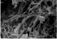
WC nanofibres Self-standing mat Fibre diameter ca. 250 nm
