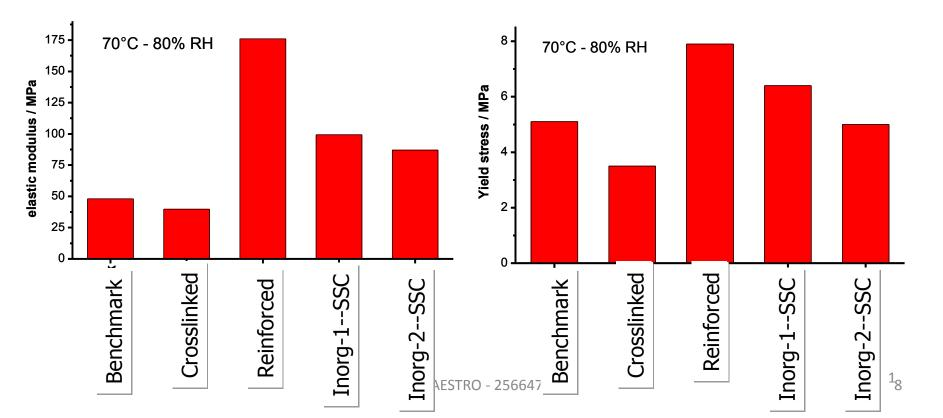
• MEAs incorporating cross-linked low EW and novel reinforced low EW SSC membranes show improved performance in *in situ* fuel cell testing at hotter, drier conditions compared to the project start point, state-of-art SSC membrane
