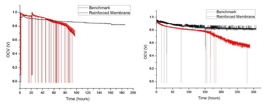
Novel reinforced low EW SSC membranes show improved MEA durability (lower voltage loss, longer lifetime) in *in situ* testing designed to accelerate chemical and/or mechanical degradation, compared to the project start point, state-of-art SSC membrane
