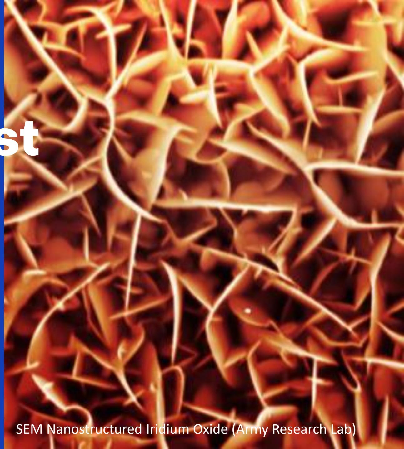
SEM Nanostructured Iridium Oxide (Army Research Lab)
