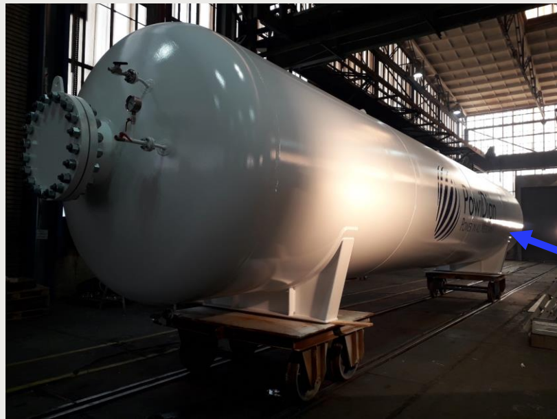
H2 tank 56m 3 / 30bars
