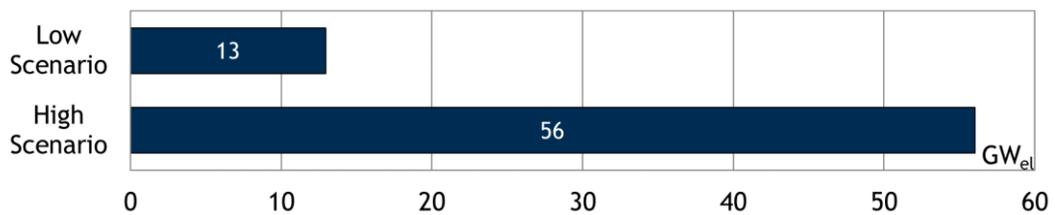
Figure 4-12 Electrolysis capacity per MS by 2030
