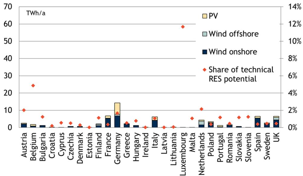
Figure 4-15 Renewable electricity input for hydrogen production per MS in the high scenario by 2030
