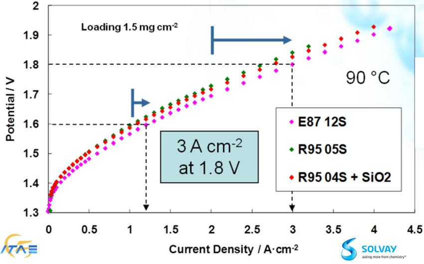
CNR-ITAE catalysts in combination with Solvay Aquivion ionomers 6
