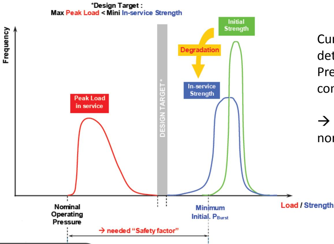
Current designs are mainly determined by Stress Ratio/Burst Pressure ratio requirement, considering **stress rupture**
