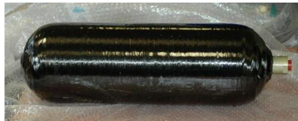
*9L cylinder especially designed for HyCOMP*
