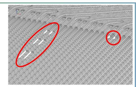
Meshed with artificially inserted obstructions
