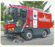
the machine was converted to run on a hydrogen fuel cell by Netherlands firm Holthausen, in cooperation with the municipality of Groningen. Finnish manufacturer Visedo supplied its expertise to electrify the vehicle's drive system.
