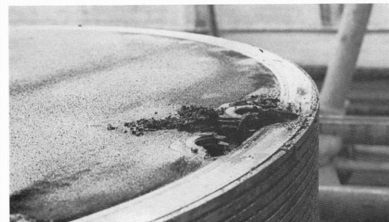
Fig 6 Cell 79 showing damage in vicinity of gas off-takes
