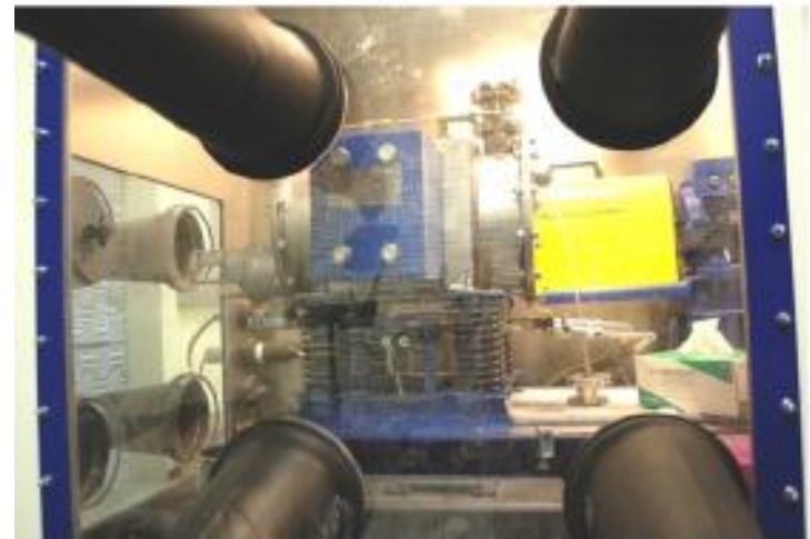
Vibrational ball mill for large scale preparation
