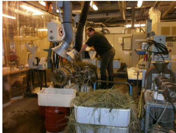
Extrusion for solid/liquid separation at circa 100 kWh/tonne dry matter
