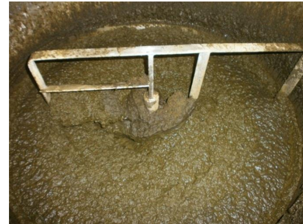
\text{Ca(OH)}_2 -pretreatment at 85-100 C, 7.5% on dry matter for increased accessibility
