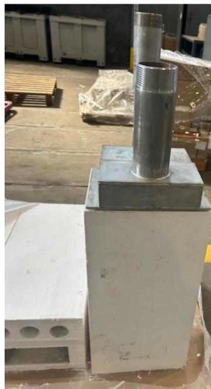
1MW burner with refractory blocks
