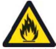
Picture 3.1.2.4-2 “Flammable material or high temperature” warning sign according to Directive 95/58/EEC
