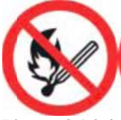
Picture 3.1.2.4-1 “No smoking and naked flames forbidden” prohibitory sign, according to Directive 95/58/EEC
