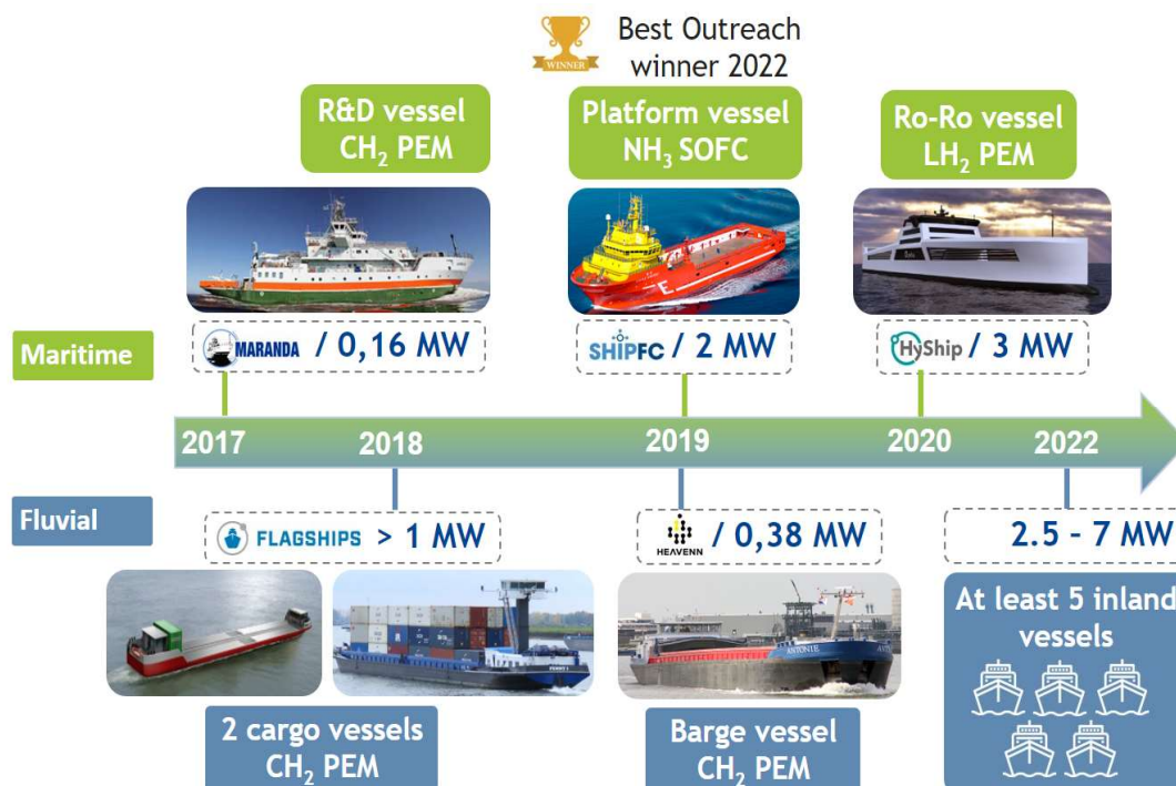
FIGURE 9. TOWARDS LARGER VESSELS AND H 2 DELIVERY BY SHIPS
