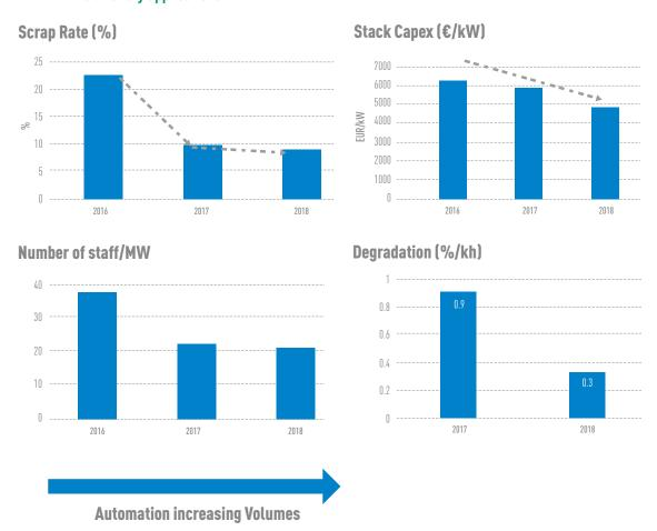
Figure 29: Improvements in selected TRUST KPIs relevant for manufacturing projects focusing on stationary applications
