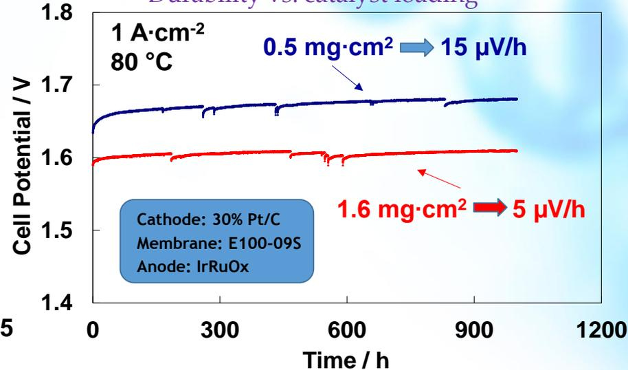
Decrease of cathode catalyst loading of 5 times did not cause significant loss
