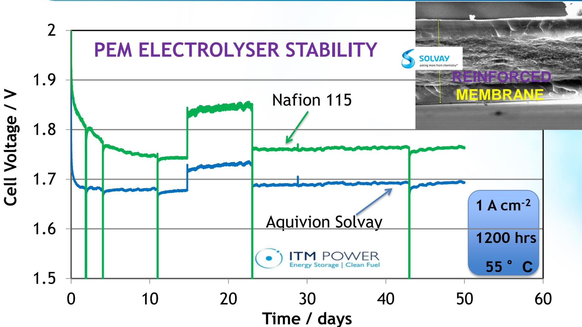
PEM electrolyser single cells containing MEAs with same catalyst loading and different membranes
