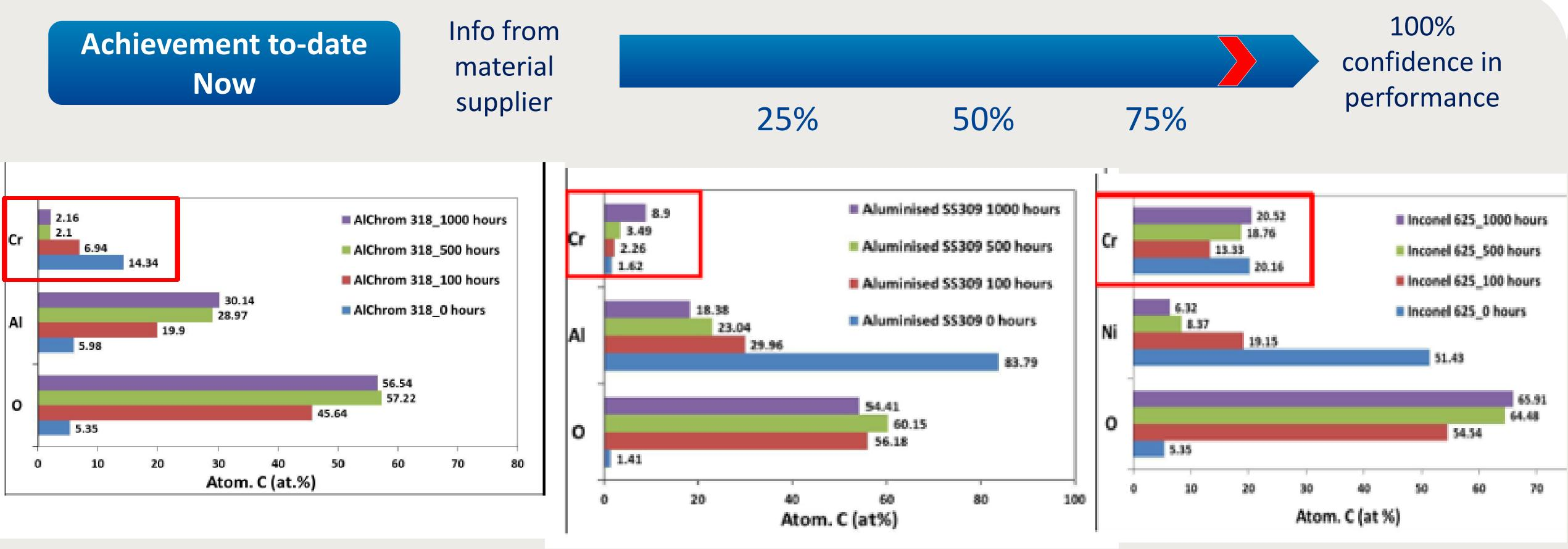
*Test Conditions:* 850 °C; 6.0 L/min Airflow; 3 vol% H<sub>2</sub>O.
