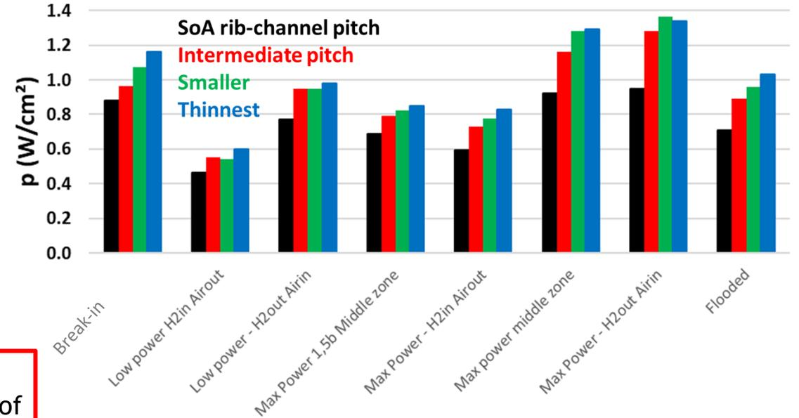
Performance for different local conditions expected in the stack: machined flow-fields with different dimensions, commercial CCM (CEA)
