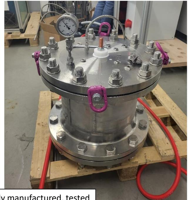
2 kW stack fully manufactured, tested and quality control completed. shipped and installed at FBK
