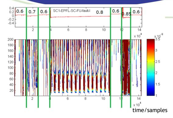
Using scale analysis technique, wavelet analysis (Continuous Wavelet Transform CWT) shows high capability to detect the **FU changes**.
