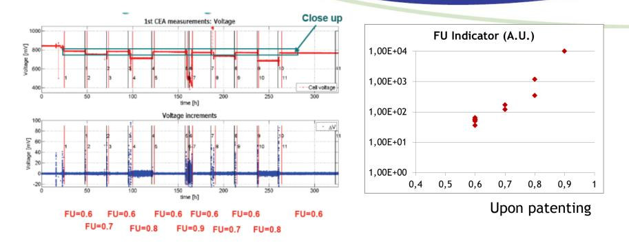
Mathematical treatment of the time varying voltage signal, shows high capability to support the **FU changes detection analysis**:
