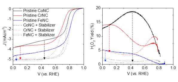
PGM-free co-catalysts have been developed that greatly reduce the side production of H<sub>2</sub>O<sub>2</sub> during ORR and improve PEMFC stability
