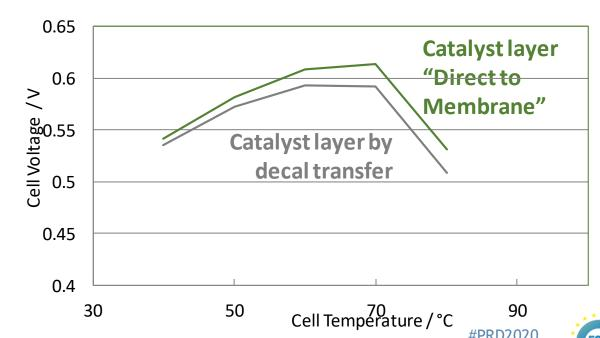
Significant improvement in performance of MEAs produced by an alternative direct to membrane coating method over a wide range of operating conditions from cool/wet to hot/dry
