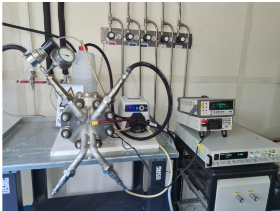
ANIONE Stack tested under differential pressure mode under horizontal configuration with KOH recirculated to the anode. KOH inlet on the bottom
