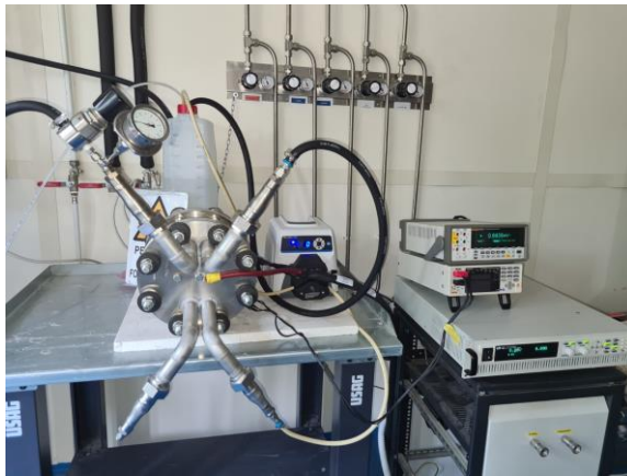
ANIONE Stack tested under differential pressure mode under horizontal configuration with KOH recirculated to the anode. KOH inlet on the bottom
