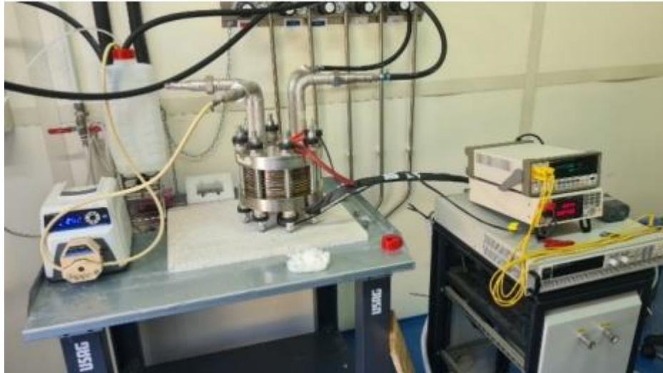
ANIONE Stack tested under ambient pressure under vertical configuration with KOH recirculated to the anode. Cell numeration
