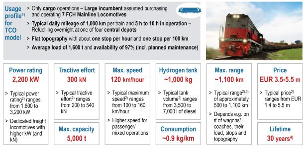
1) Duty cycle data from FINE D3.1 based on EN 50591 2) For diesel locomotives recently purchased in main European markets 3) Based on tank volumes and average considered speed; 0.25 liters of fuel per kilowatt hour 4) Potentially replacement of fuel cells or parts of it necessary after certain period Source: Expert interviews; Market research; Roland Berger
