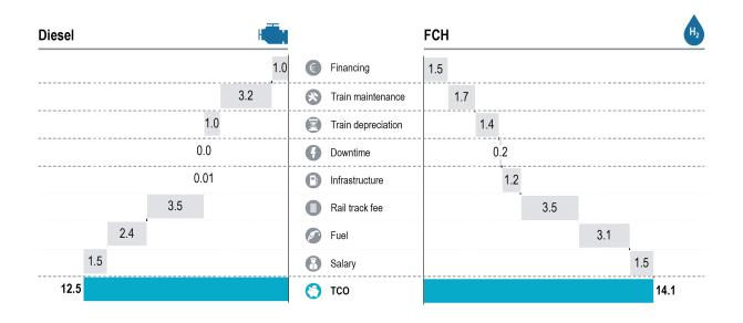
Figure 14: Detailed TCO - Shunter in base case [EUR/km]
