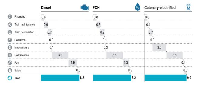
Figure 20: Detailed TCO - Multiple Unit in base case with H2 being purchased externally [EUR/ km]
