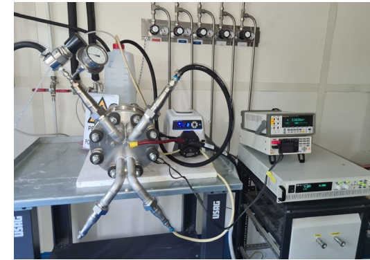
Differential pressure Horizontal Stack, anode feed 1 M KOH, flow 0.5 l/min
