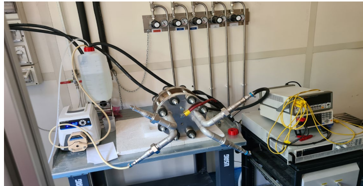
Horizontal Stack, anode feed 1 M KOH, flow 0.5 l/min
