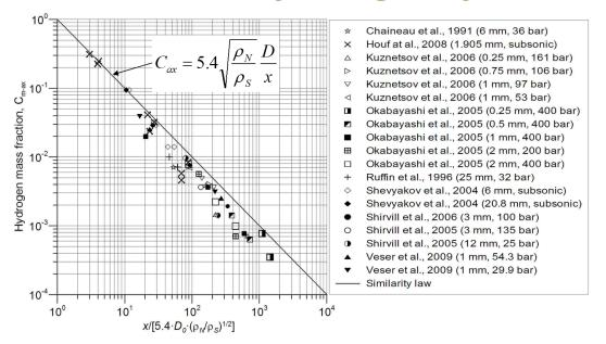
Hazard distance, i.e. the flammable envelop size (up to LFL=4%), is proportional to the leak diameter. Conclusion: decrease a pipe diameter as much as possible.
