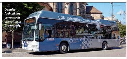
Bozen and Milan (IT), London (UK), Oslo (NO), Whistler (CA), Cologne and Hamburg (DE). The only tailpipe emissions from these vehicles is water vapour and when fuelled with hydrogen from renewable sources, the buses achieve high well-to-wheel CO<sub>2</sub> emission savings: **the buses** have saved nearly 4.5 million litres of fuel and over 6,000 tonnes of CO, to date.
