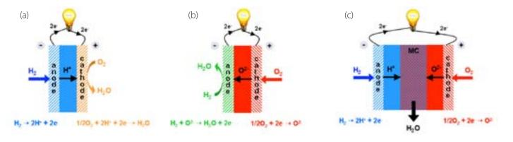
Figure 1: Scheme of (a) a PCFC, (b) a SOFC and (c) the IDEAL-Cell concept.
