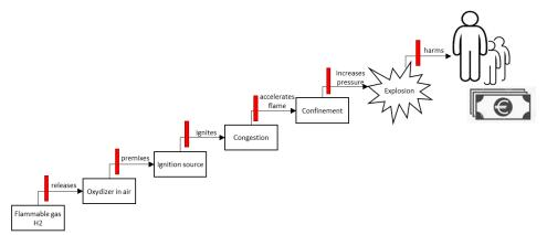
Figure 4-3: Example of escalation path in a gas explosion incident with potential barriers indicated as red barriers.
