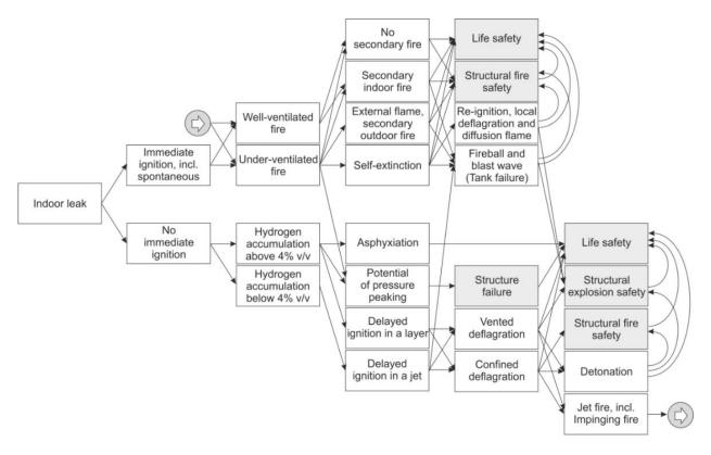
Figure 4-2. Phenomena and consequences diagram for indoor use of hydrogen.
