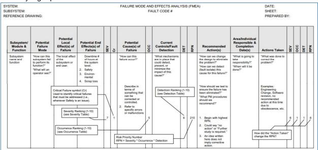
Figure A4-3: Example for an FMEA worksheet.
