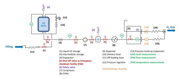
Figure A6-1: Schematic components of a Hydrogen fuelling station with liquid H2 supplied using a tank car (adapted from P.G.J.Timmers and G. Stam ICHS 2017)
