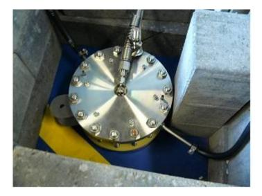
Results: A circular cell design Active electrode area: 69 cm<sup>2</sup> 29 cells Nominal operating: Input voltage 48 V Input stack current of 83 A
