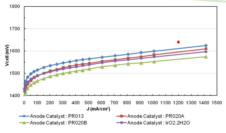
IR-corrected polarization curves @ 6 bar, 70°C,  $\lambda$ =10
