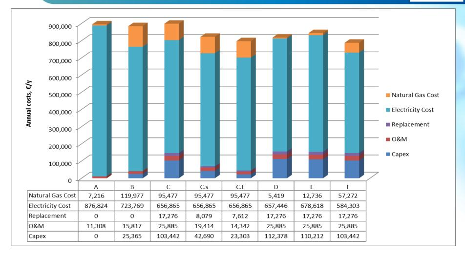
**A**: boiler - **B**: mGT - **C**: SOFC (C: current scenario, C.s: short term scenario, C.t: target scenario) - **D**: SOFC with centrifugal pre-thickening - **E**: SOFC with dynamic pre-thickening - **F**: SOFC (UK)
