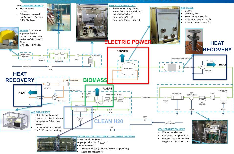
Proof-of-concept SOFC-based poly-generation system (biogas - SOFC CHP - C recovery - waste water cleaning): designed, built, tested indoor DEMO in real WWTP industrial site for 6 months: end @ April 30th, 2015
