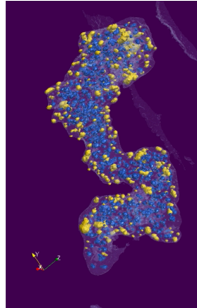
AFM: 3D height-image with superposed stiffness values
