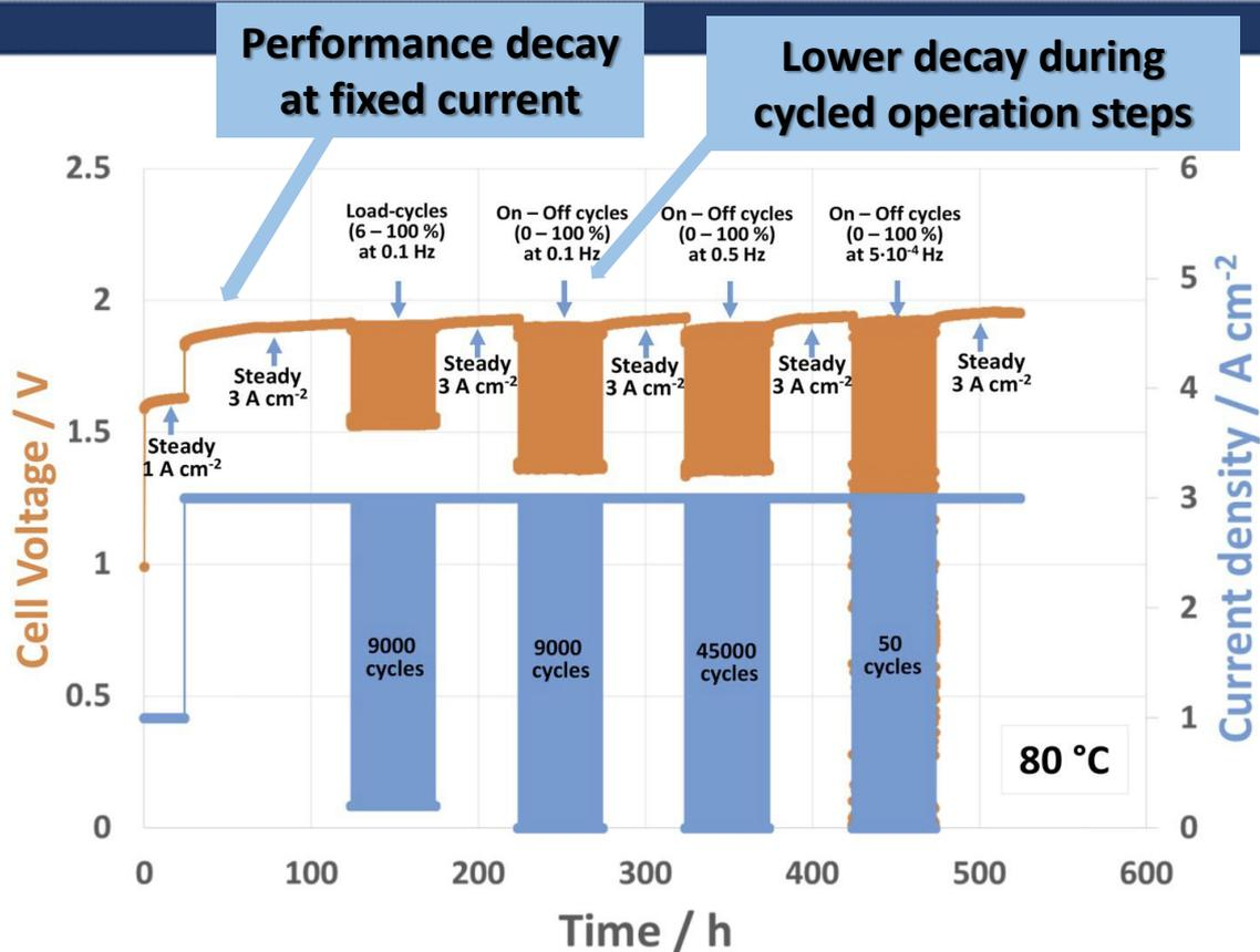
➤ A periodic decrease of the operating current density can mitigate performance losses by producing only a recover of reversible degradation
