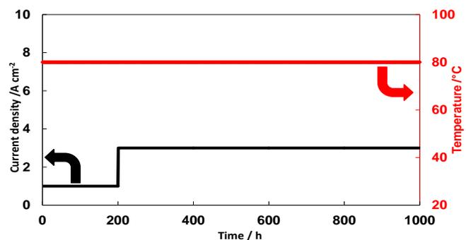
MEA durability test: steady-state
