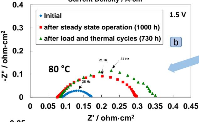
Increase of R<sub>p</sub> → catalyst degradation
