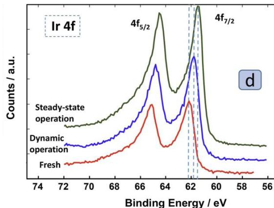
Shift to lower B.E. in the used sample → Ir<sup>4+</sup> to sub-stoichiometric Ir<sup>3+</sup>
