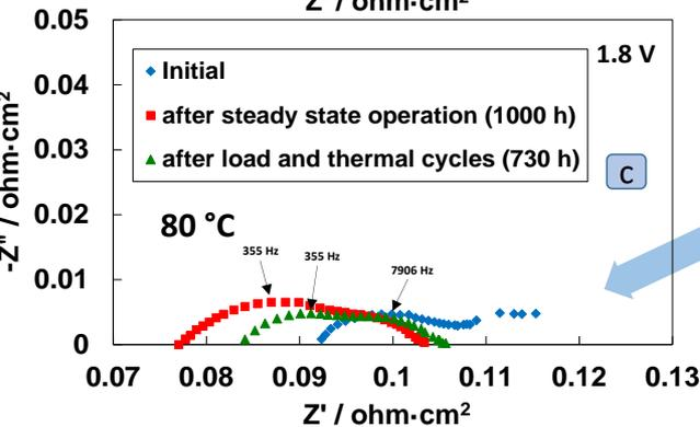
Reduction of R<sub>s</sub> → cleaning and/or thinning of the membrane
