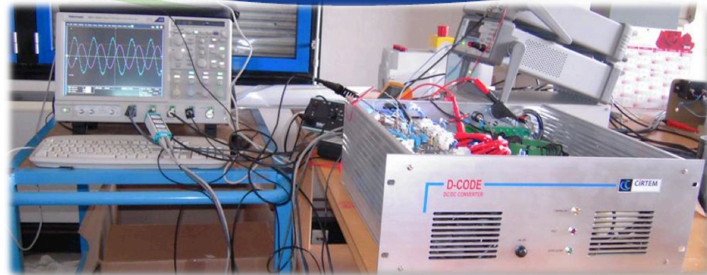
HV DC/DC converter under testing
