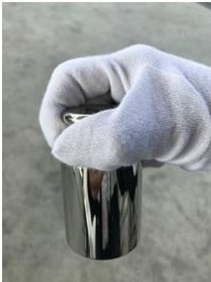
Figure 3: Calibrated weights handled cautiously with gloves
