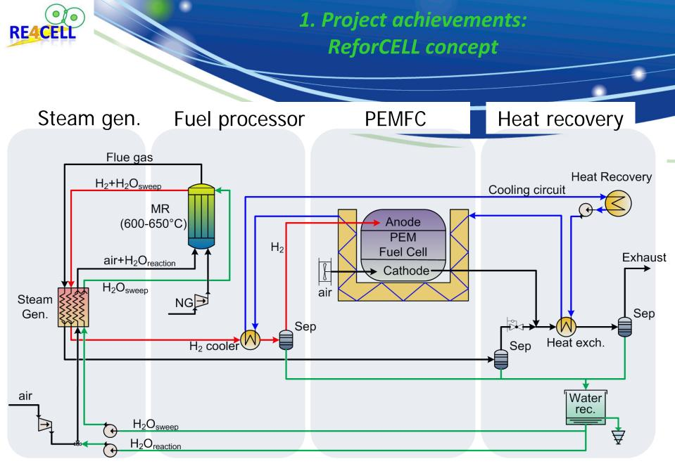
PEM m-CHP unit using catalytic membrane reactor for fuel processing Programme Review Day 2012 – Brussels, 28 & 29 November 2012 Pág. 5
