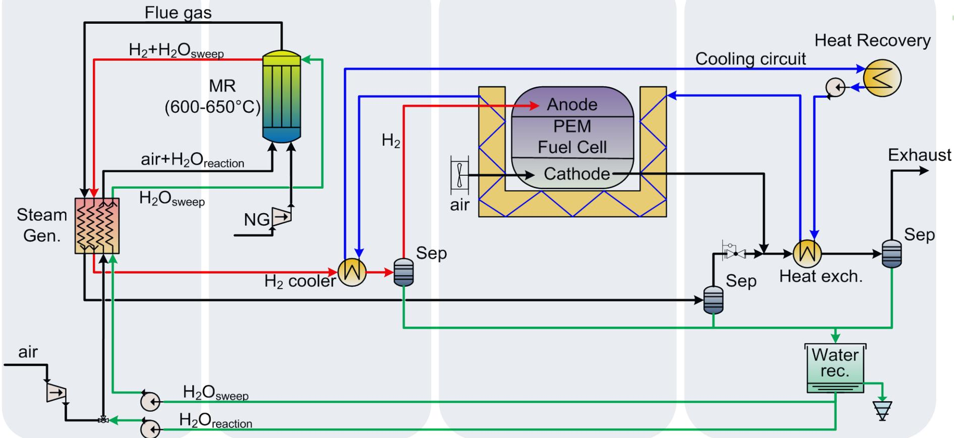
PEM m-CHP unit using catalytic membrane reactor for fuel processing
