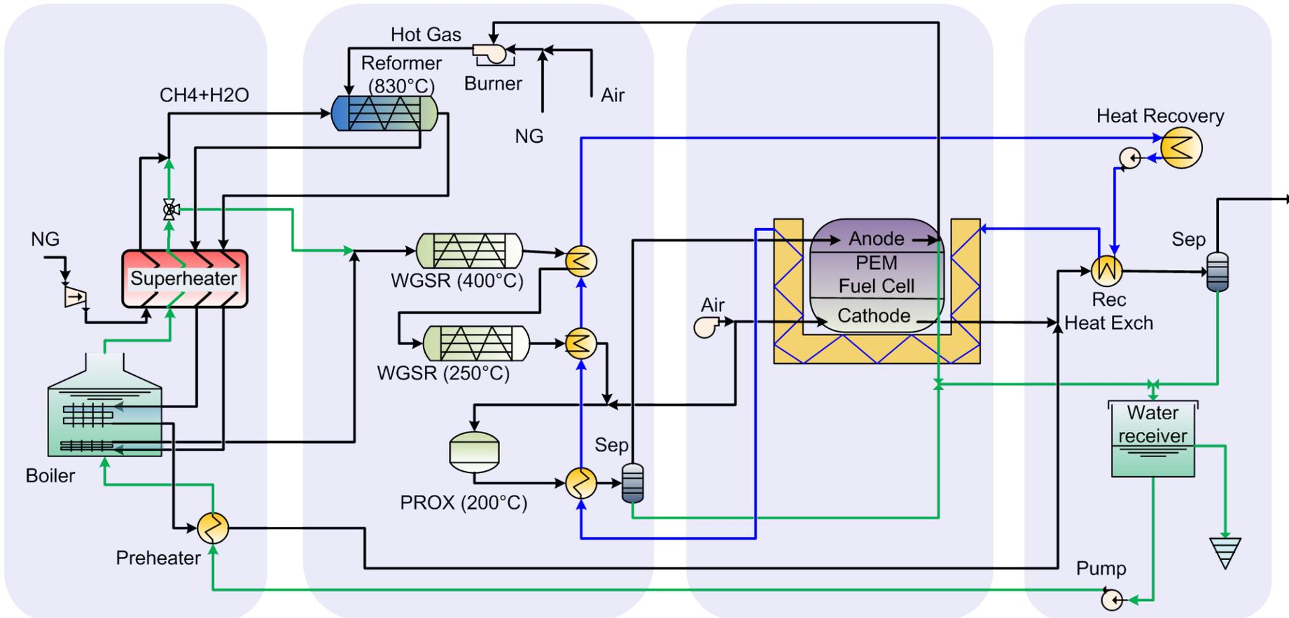
PEM m-CHP unit using traditional reforming for fuel processing
