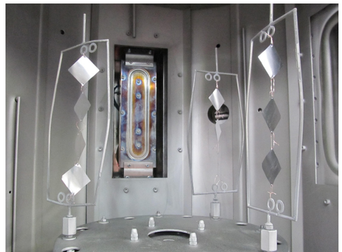
Linear Ion Source cleaning of substrates.
