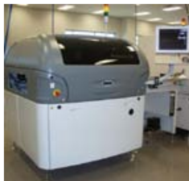
Screen printing machine to manufacture controlled active layers
