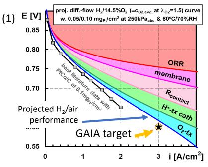
Best literature data<sup>1</sup> (grey (2) dots/line) data under comparable conditions (94°C/65% RH, 250 kPa<sub>abs</sub>,  $\lambda_{H2}/\lambda_{air} = 1.5/2.0$  at anode/cathode loadings of 0.05/0.10 mg<sub>Pt</sub>/cm<sup>2</sup>) do not reach GAIA target
