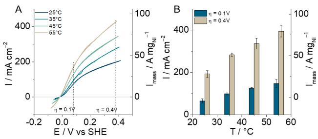
Target current density with non-PGM anode at 0.1 V was exceeded by a factor 2 at 55 °C
