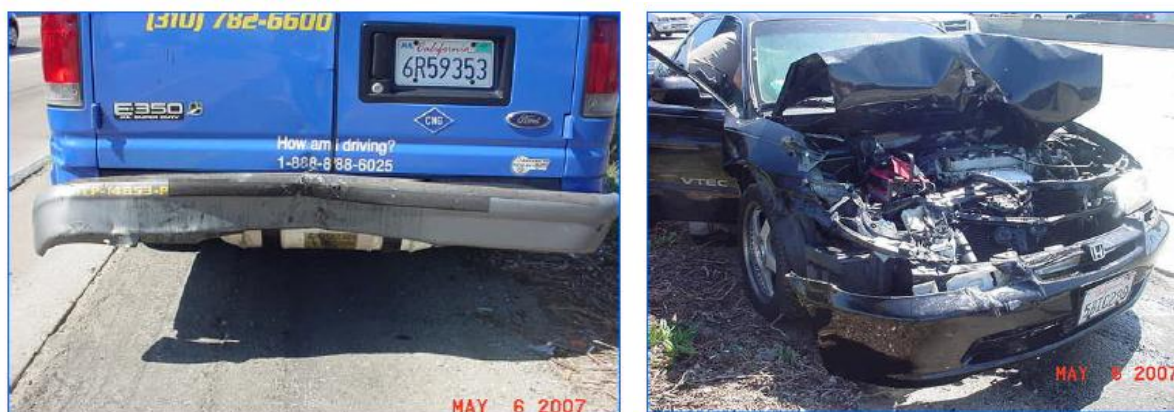
Figure 3.26. Ford van damage (left) and Honda Accord (right) damage after rear impact accident.
