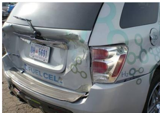
Figure 3.14. FCEV Chevrolet Equinox involved in accidents during the 'Project Driveway' demonstration project
