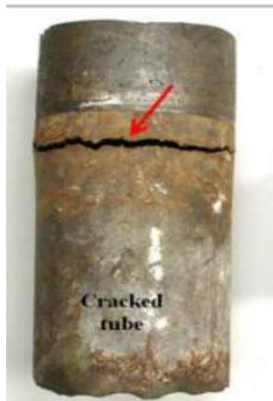
Figure 1.2. Crack formed on a plant tube.
