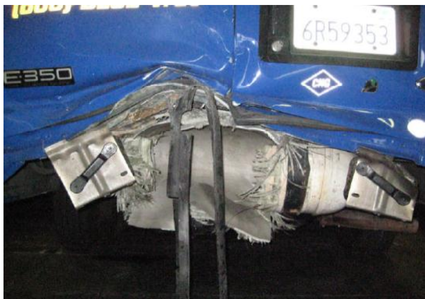
Figure 3.27. The rear van tank after the burst.
